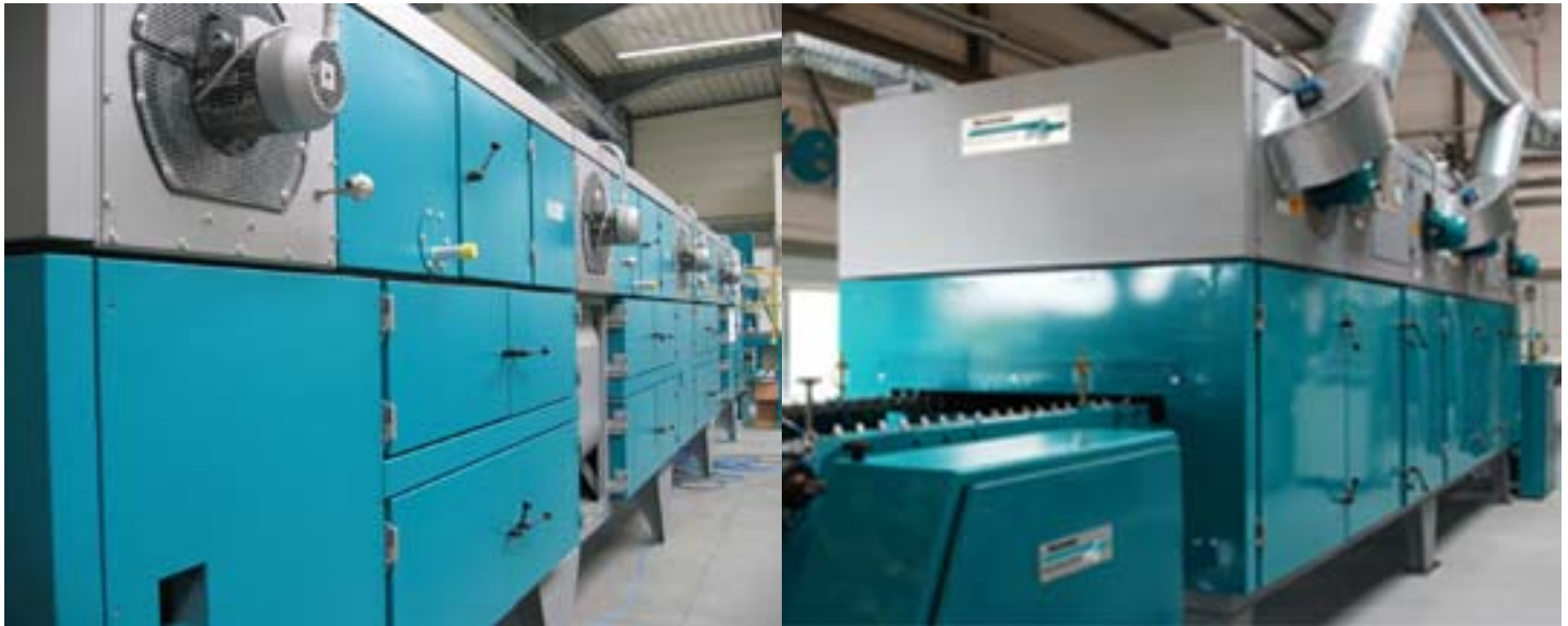
For complex tasks each 3 meter Coatema Moduldry section is fitted with an exhaust ventilator.
