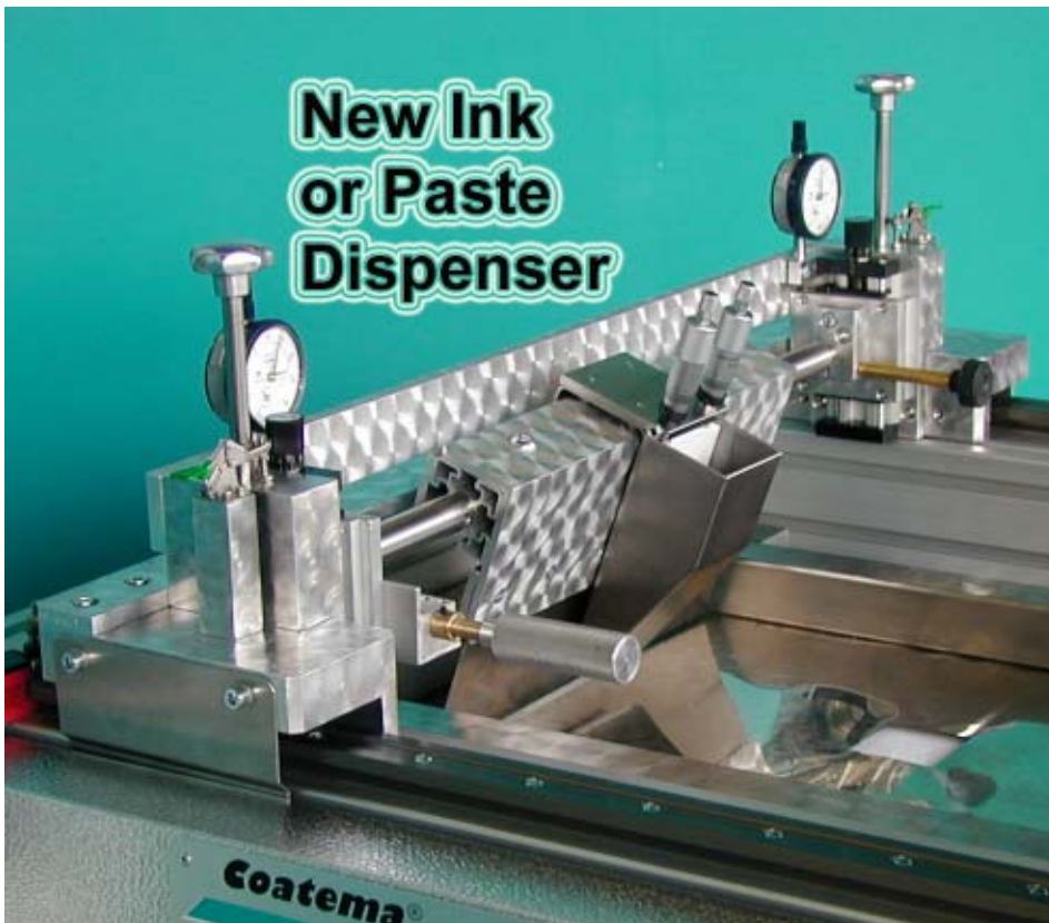
New dispenser is adjustable in gap and angle with a precision gauges.
