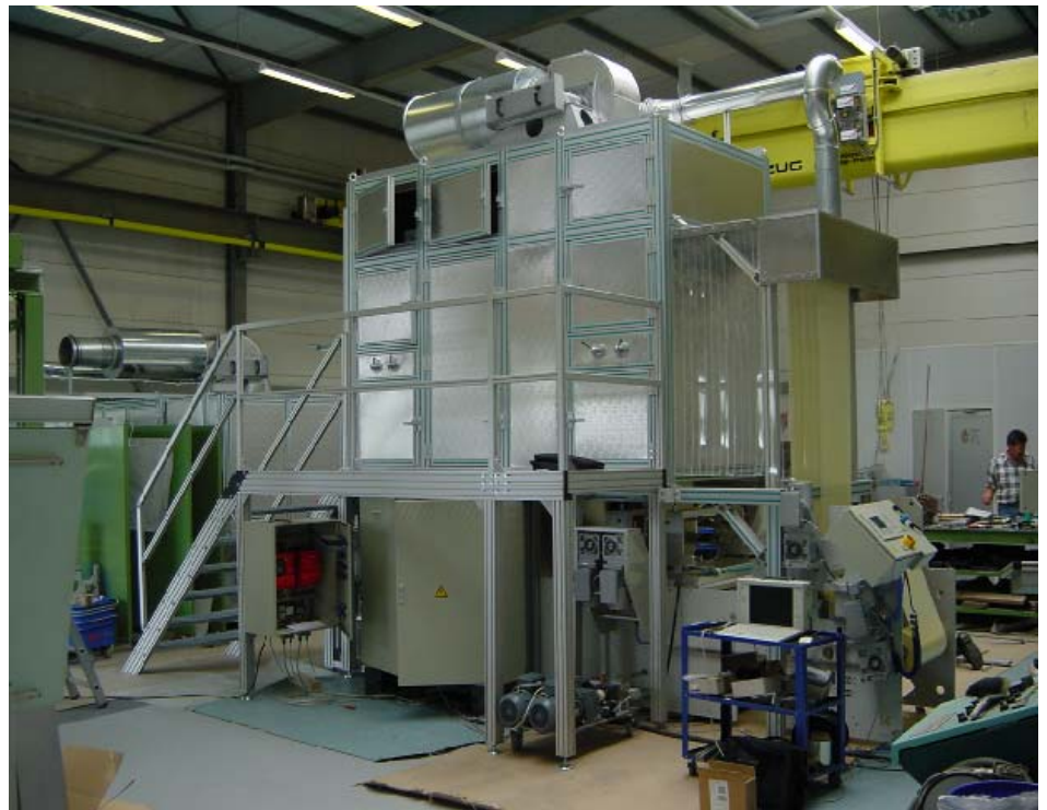
The Verticoater 500-1000, from Coatema Maschinenbau GmbH, is a double-sided vertical coating, drying and calendering systems currently in use for LiPoBat components.
