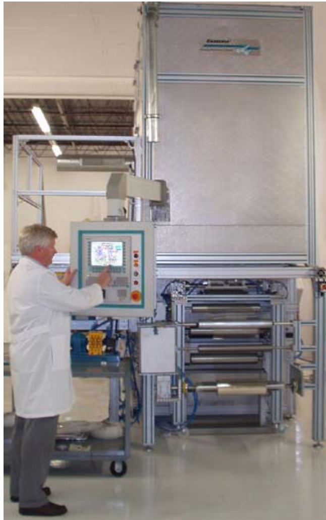
Dr. Mark Daroux, CTFC R&D Director, selects casting parameters for vertical simultaneous two-sided slot-die coating for thin film renewable energy cell elements using a new Coatema Verticoater 500.
